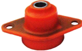
SOPORTE P/ CABINA KENWORTH, INTERNATIONAL TRUCK EXT. 3 3/8" INT. 25/32" ALT. 3" HO. 17/32
