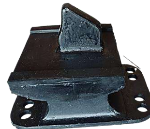
SOPORTE P/SUSPENSION DELANTERA FREIGHTLINER ALT. 3" ANCHO 2 7/8" LG. 4 3/8"
