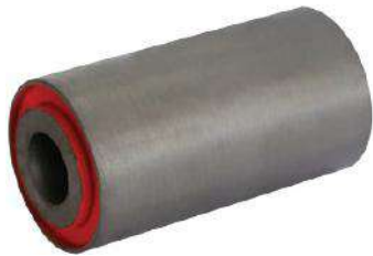
BUJE P/ MUELLE FREIGHTLINER CENTURY/CASCADIA. EXT. 2 1/4" INT. 3/4" LG. 4 1/4"
