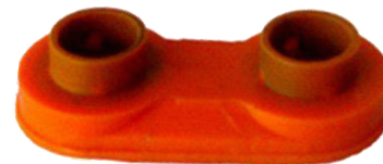
SOPORTE DELANTERO P/MOTOR FREIGHTLINER LG. 7 1/4" ANCHO 3 1/4" INT. 3/4" C.C. 4"
