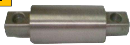
PERNO P/BARRA FREIGHTLINER EXT. 1 3/4" BARR. 21/32" C-C 5 3/8" LG. 6 3/8"
