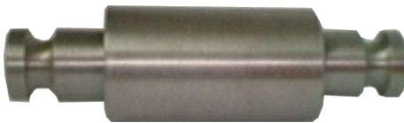
PERNO MUELLE DELANTERA KENWORTH EXT. 2 5/64" EXT.< 1 1/16" C.C. 6 5/16 LG. 7 1/2 "
