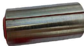
BUJE MUELLE DELANTERA KENWORTH (2012-2013) EXT. 1 3/4" INT. 5/8" LG. 4 1/4"
