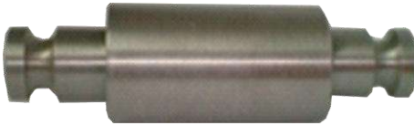
PERNO MUELLE FRONTAL KENWORTH EXT. 1 3/4" EXT.< 1 1/16" C.C. 5 7/16" LG. 6 5/8"
