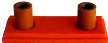
SOPORTE TRASERO P/MOTOR FREIGHTLINER LG. 6 9/16" ANCHO 2 9/16" INT. 25/32" C.C. 4"
