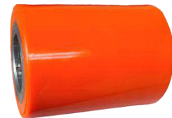
BUJE P/TENSOR UNIVERSAL EXT. 1 15/16" INT. 7/8" LG. 3"
