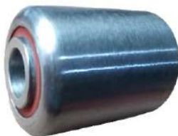
BUJE LATERAL P/MUELLE SUSPENSION HENDRICKSON E-4. EXT. 2 3/8" INT. 1" LG. 3 1/8"
