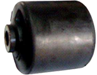
BUJE TRIDIFUNCIONAL P/SUSP. HENDRICKSON EXT. 5 15/16" INT. 1 1/4" LG. 6 3/4
