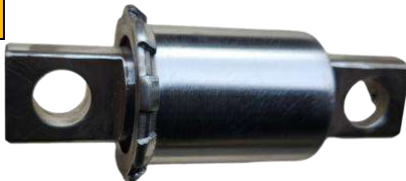
GRANADA P/SUSPENSION FREIGHTLINER, FAS II AIRLINER/FL EXT. 2 1/2" C-C. 5 11/16" HO. 13/16"
